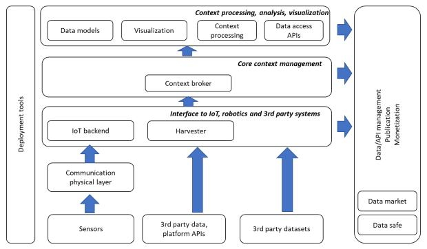
Figure 2. Typical architecture for a Big Data platform applied to the water sector. An interrelation of the elements is shown: Devices/data sources, connectivity/network, data framework intelligence framework and data market.
