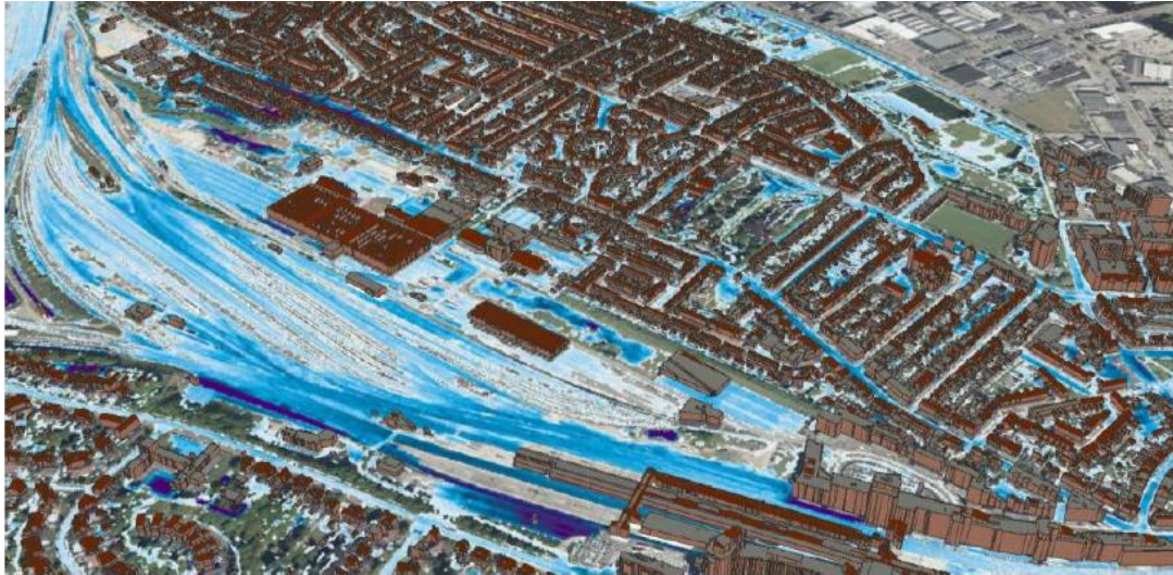
Figure 2: Visualisation provided by the hydrological model displaying the expected flooding resulting from a certain amount of precipitation (160mm in 2 hours) occurring in the Soesterkwartier-neighbourhood 3
