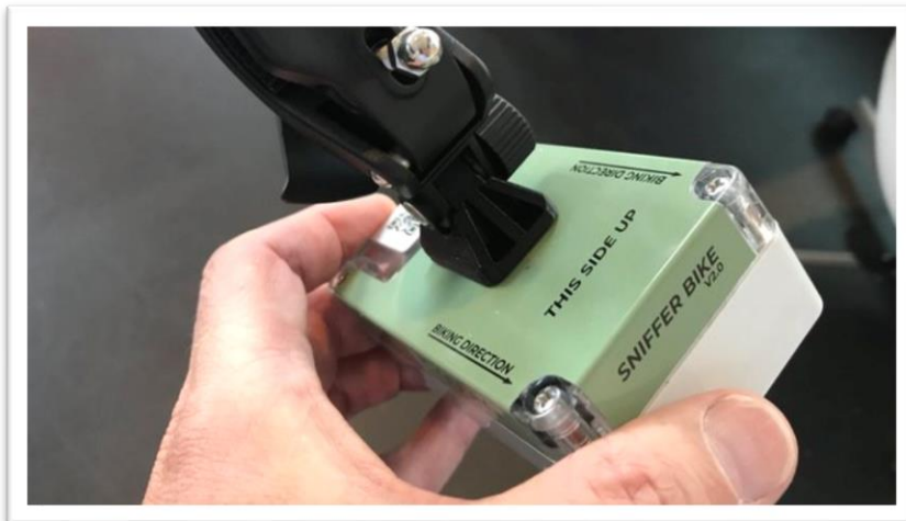
Figure 4 The current Snifferbike sensor for measuring air quality and cycle routes
